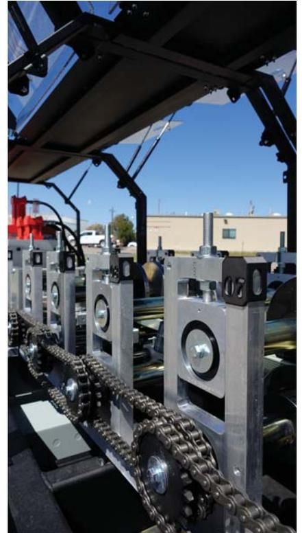
KFD-2025E Non-Structural Stud and Track Machine. PHOTOS COURTESY OF KNUDSON MFG.
