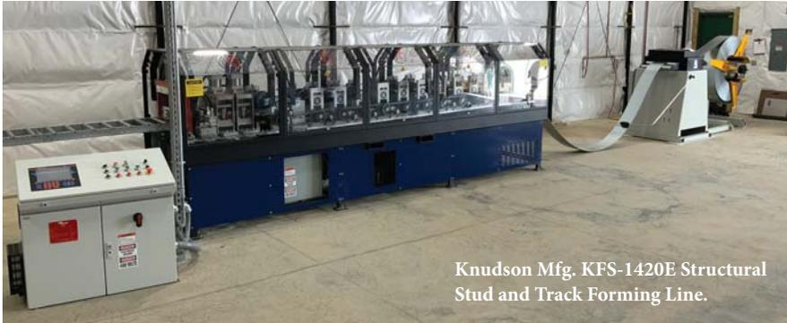
Knudson Mfg. KFS-1420E Structural Stud and Track Forming Line.
